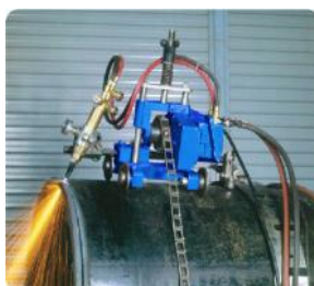
Cutting edge sharp = V 0 - 45°
