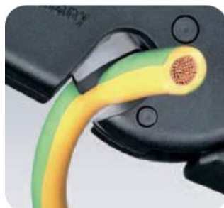
Integral Wire cutter, max.10 mm 2
