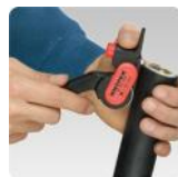
Setting the tool or longitudinal cut
