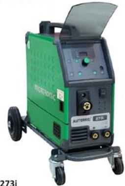
Automig 2 273i 205 A , 100 % , 3 Phase Max. wire dia. 1.0 mm IGBT Module Inverter
