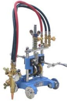
KC - 11 Hand Pipe Gas Cutting Pipe Cutting Dia. 100 - 600 mm Pipe Cutting Thickness 5 - 50 mm
