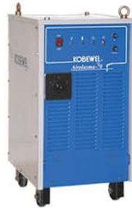
Air Plasma 70 70 A , 60 % , 3 Phase 3 Cutting steps, 30 - 50 - 70 A Max. cut 25 mm Rectifier Technology
