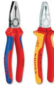
Combination Pliers Cut. Hard Wire \varnothing : 2.0 - 2.5 mm Cut. Cable \varnothing : 10.0 - 13.0 mm Cut. Cable Section 16.0 mm 2
