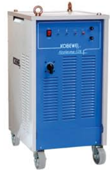
Air Plasma 120 120 A , 60 % , 3 Phase 4 Cutting steps, 30 - 60 - 90 - 120 A Max. cut 45 mm Rectifier Technology
