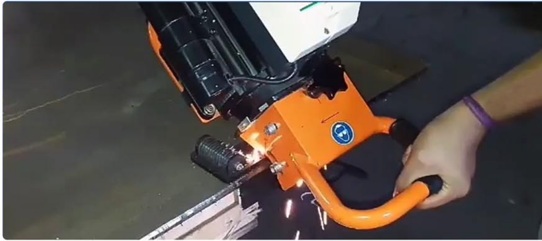
Beveling Machine SKF 63 - 15 1.100 Watt Bevel width : 15 mm max.
