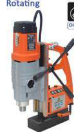
Rotabest 100 RL-E Core Drill max. Ø 100 mm Twist Drill max. Ø 32 mm 2.500 watt 110 - 175 - 245 - 385 RPM
