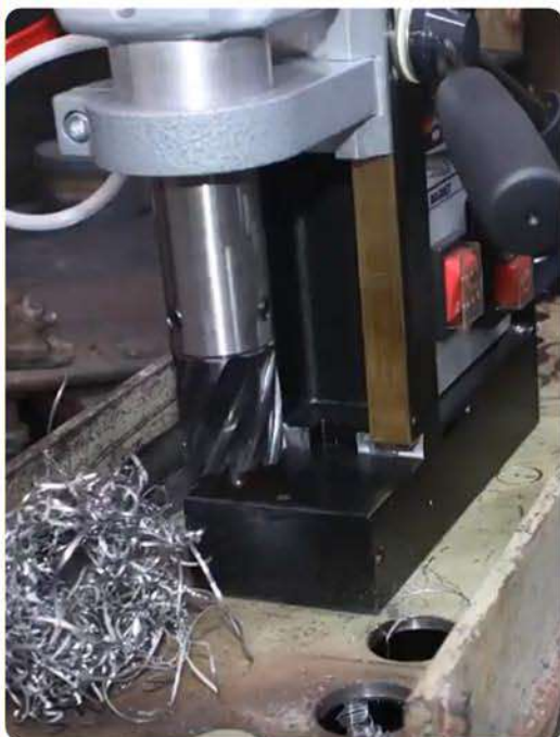
HSS Cobalt Blue, Depth 30 Ø 12 - 40 mm Weldon Shank
