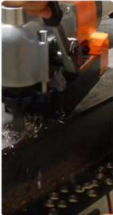
Rotabest 80 X Core Drill max. Ø 80 mm Twist Drill max. Ø 32 mm 1.800 watt 110 - 175 - 245 - 385 RPM
