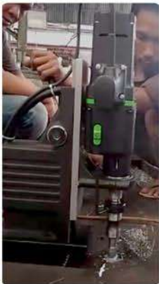
MD 300 N Semi Auto Core Drill max. Ø 30 mm 1.100 watt 550 - 330 RPM
