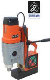
Rotabest 80 X Core Drill max. Ø 80 mm Twist Drill max. Ø 32 mm 1.800 watt 110 - 175 - 245 - 385 RPM
