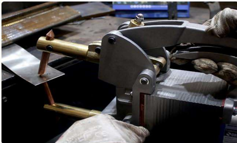
DAIICHI Japan Portable Spot Welding
