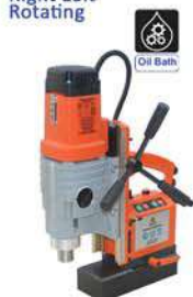
Rotabest 60 RL-E Core Drill max. Ø 80 mm Twist Drill max. Ø 32 mm 1.800 watt 110 - 175 - 245 - 385 RPM
