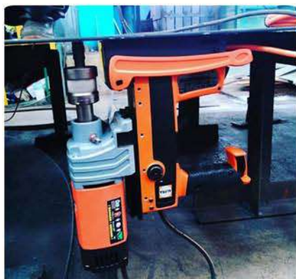
Rotabest RB 35 SP Core Drill max. Ø 35 mm 1.100 watt 450 RPM
