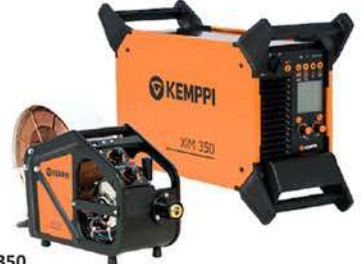
Xim 350 350 A, 60 %, 3 Phase Max. wire dia. 1.6 mm IGBT Inverter
