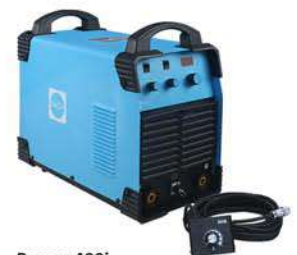
Power 400i 400 A , 60 % , 3 Phase Digital Display, Arc Force Remote Control, IGBT Module Inverter
