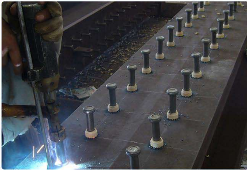
RSN 2500 II Stud Welding Welding Range : 200 - 2500 A Stud Range : 10 - 25 mm 3 Phase
