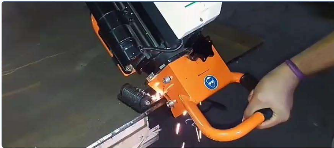
Bevelling Machine SKF 63 - 15 1.100 Watt Bevel width : 15 mm max.
