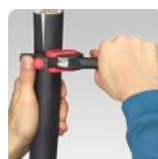
Turning the tool for circumferential cut
