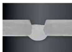
IAC root pass welded in vertical downwards position in 5 mm mild steel.
