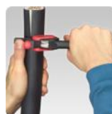
Turning the tool for circumferential cut
