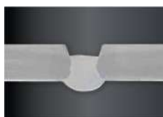
IAC root pass welded in vertical downwards position in 5 mm mild steel.
