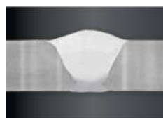
IAC root pass welded in vertical downwards position in 10 mm mild steel, filled with two Sequence Repeat passes in vertical downwards position.
